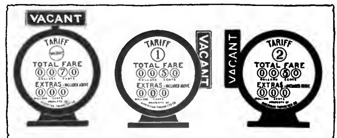
Fig. 3—Three positions of the flag. At the left is the position when the cab is vacant, in the center is the position for tariff 1 and at the right for tariff 2
